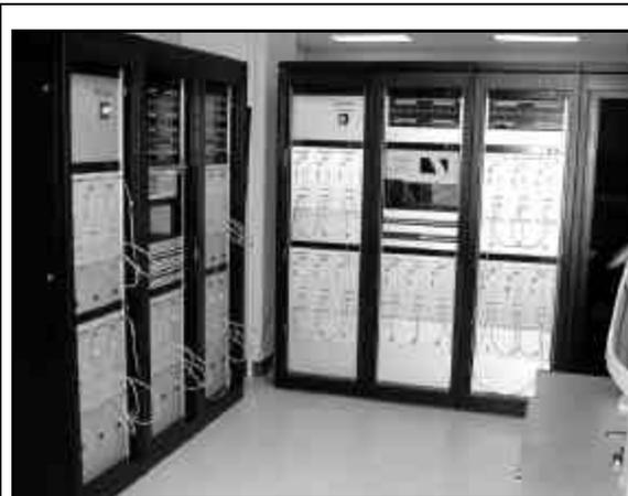
Figure 1: 30 nodes digital real time simulator
