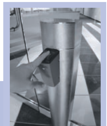
Figure 2 (right): Biometric verification methods ensure that the person is actually who he/she claims to be. Shown here is a fingerprint scanner at a TELUS intelligent Internet Data Centre.
