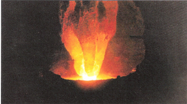
Figure 3: Arcing electrode tip in a furnace
