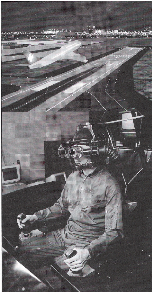
Figure 1: CAE's Computer image and helmet mounted display for flight simulators
