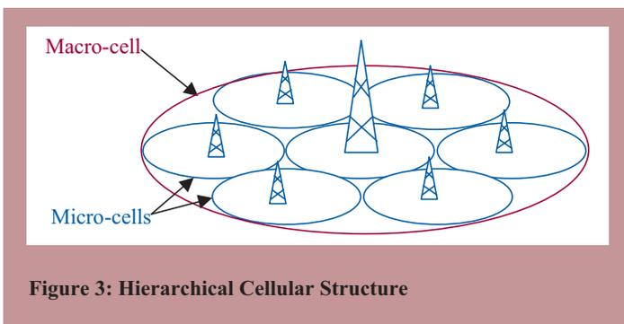
Figure 3: Hierarchical Cellular Structure
