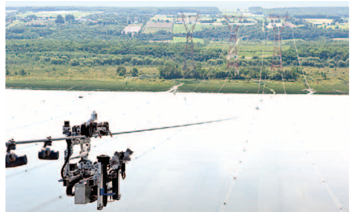
LineScout deployed in 735 kV powerline inspection over a large water crossing
