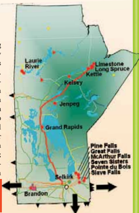
Figure 1: Existing Generation and Major Transmission System
