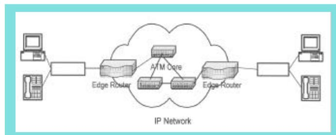
Figure 3: Delay-sensitive traffic channeled to ATM core
