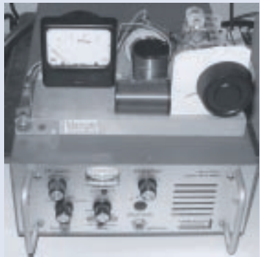
Figure 1: (Top) Prototype receiver. The aerial is inductively coupled to the first of three capacitively coupled tuned circuits. The output is taken from the third stage and detected with a geranium diode in half wave mode. The meter measures micro-amps and is in series with the headphones. (Bottom) The Marconi XH-100 superheterodyne receiver used in the re-enactment.
