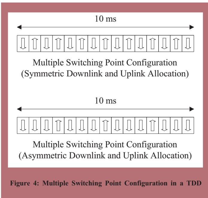
Figure 4: Multiple Switching Point Configuration in a TDD
