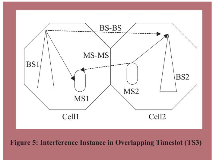
Figure 5: Interference Instance in Overlapping Timeslot (TS3)
