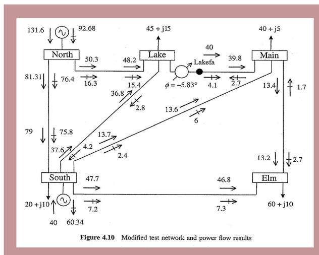
Figure 4.10 Modified test network and power flow results
