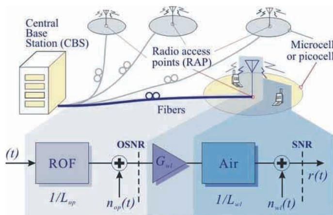
Figure 1: ADROIT fiber-wireless solution for cellular radio networks
