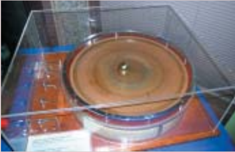
Tesla Exhibition: Tesla's induction motor with egg shaped rotor called "Columbus' Egg". Photo courtesy of Ana Ristic.
