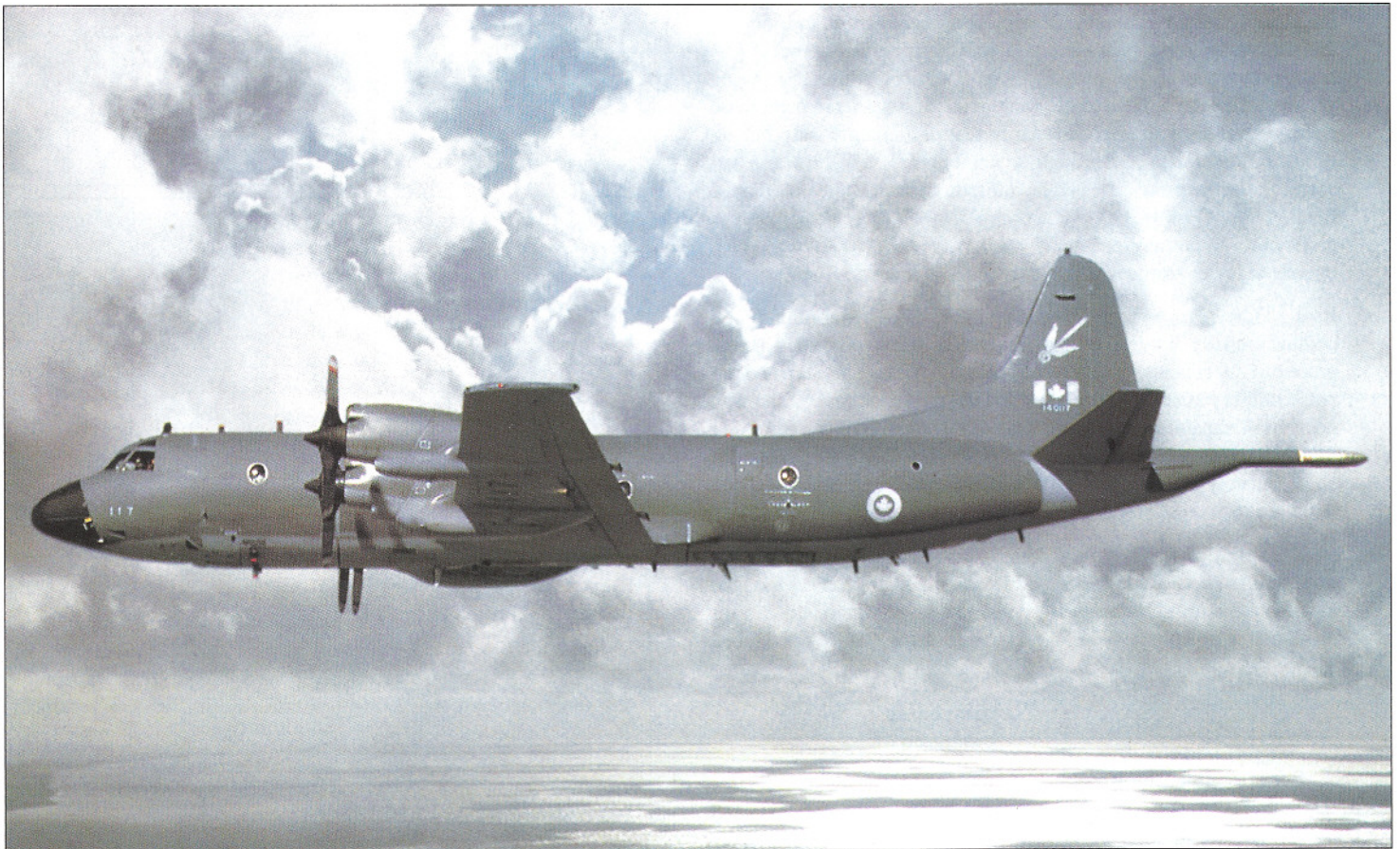
Figure 3: The CP-140 Aurora Maritime Patrol Aircraft. Canada's fleet of Auroras will be upgraded with the Spotlight SAR system under the Aurora Life Extension Project.
