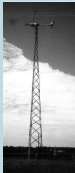
Figure 9: Bergey Excel 10 kW wind turbine for inverter research and development.
