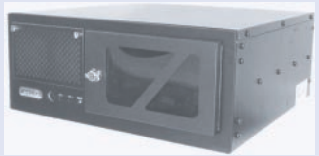
Figure 11: Multi-processor Electrical Engineering Simulator, an industrial-quality unit equipped with three 1 GHz CPUs (expandable to 5 by adding one dual-CPU board). The CPUs communicate via shared memory, and multiple units can be linked via FireWire to assemble a mega-simulator.
