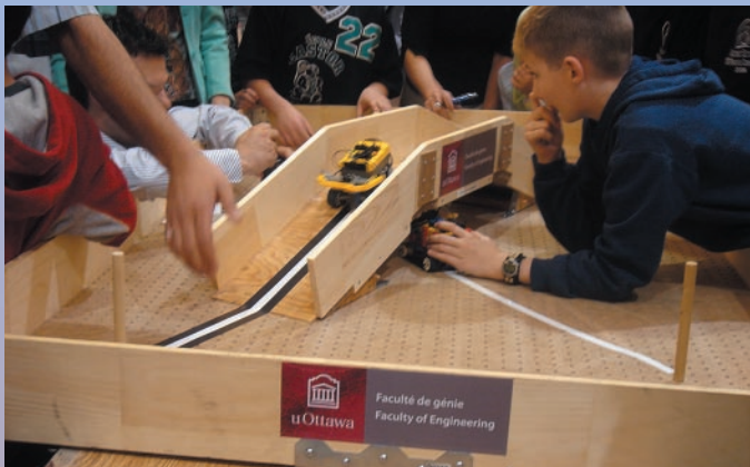
The Goulbourn Middle School’s Linebot3 team calibrates their light sensor in preparation of their timed run through the junior challenge. The junior teams found out that the shadow under the bridge needed to be accounted for, as it differed from the values they obtained with their own school mockups.
