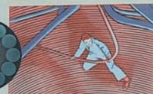
A worker leads the TAT-1 cable in the hold of the Monarch, as the ship prepares for the journey across the North Atlantic. The Monarch was the largest cable ship afloat at that time with four cable holds each 270 feet in diameter.
