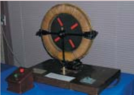
Tesla Exhibition: Model of Tesla's induction motor with disk shaped rotor. Photo courtesy of Ana Ristic.
