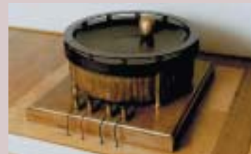
Tesla exhibited this ingenious model of the induction motor (rotor is a freely rotating metal egg) at the Chicago World Exhibition, 1893. Photo courtesy of Tesla Museum, Belgrade.
