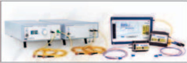
Figure 5: Various high performance erbium-doped fibre (EDF) instruments (amplifiers, broadband sources, comb sources) and amplifiers developed and manufactured by MPB.
