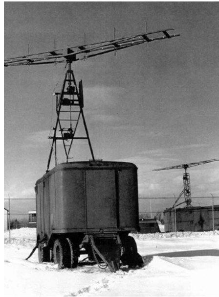
The Zone Position Indicator (ZPI) unit of the GL III (c) spotted targets. The design was adapted from earlier British systems.
