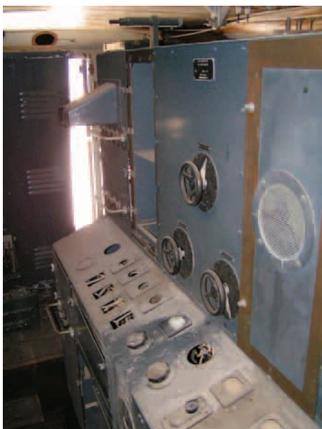
The interior of the Zone Position Indicator (ZPI) cabin of the GL III (c) on display at CFB Shilo. Photo Credit: CARA.
