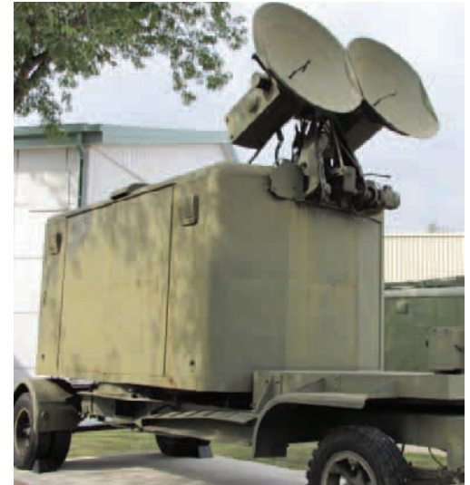
The Accurate Position Finder (APF) trailer of the GL III (c) gunlaying radar system on display at the Royal Canadian Artillery Museum at CFB Shilo, Manitoba. Photo Credit: Cal Gibson.
