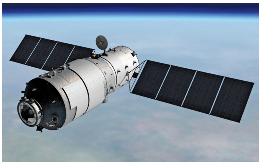
Figure 1: China’s Tiangong-1 space station. The main cylindrical body was 10.4 m long and had a 3.35-m diameter, comparable in volume to a school bus. (Source: China Manned Space Engineering Office.)
