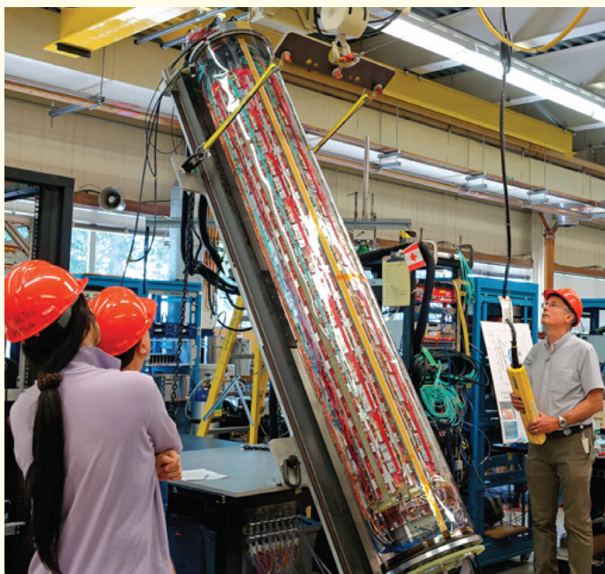
Scientists at TRIUMF position the ALPHA-g detector in preparation for testing. The instrument was shipped in July 2018 to CERN, which is the only facility that can produce antimatter in sufficient quantity for the experiment. (Source: Stu Shepherd/TRIUMF.)
