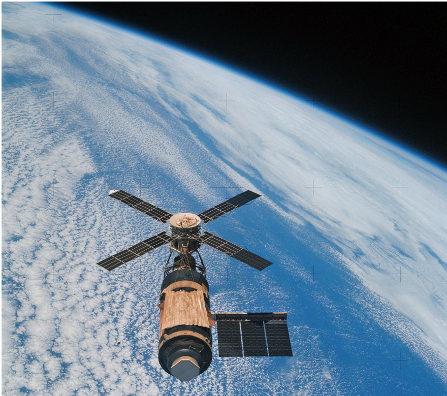
Figure 4: The U.S. Skylab space station. The main cylindrical body was 25.1 m with a 6.6-m diameter—a volume an order of magnitude larger than that of Tiangong-1 . During the 1973 launch, a micrometeoroid hit the station, jamming one of the main solar panels before it could be deployed. The crew was able to recover and use the station as shown until its decommissioning in 1979. (Source: NASA.)
