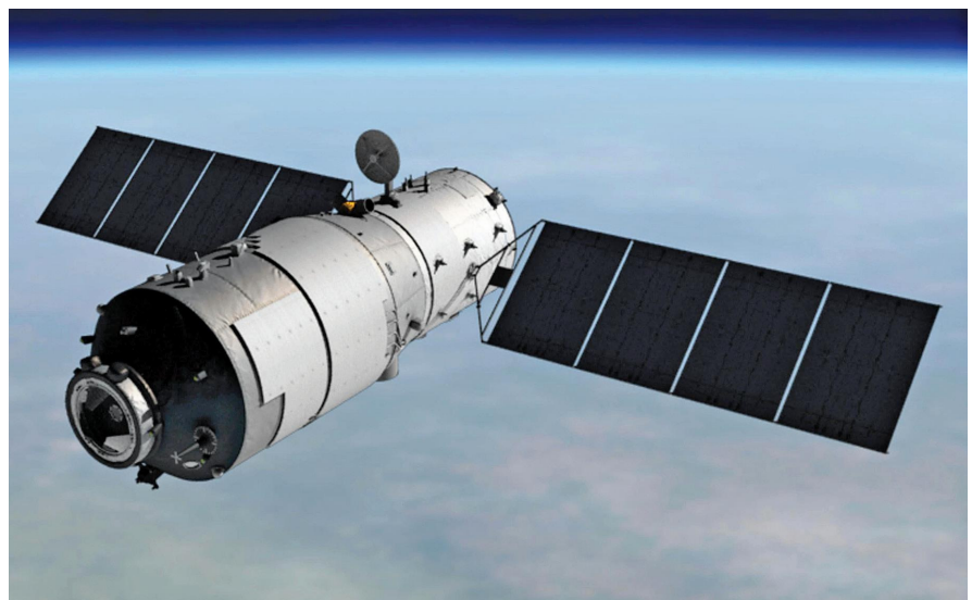
Figure 1: China's Tiangong-1 space station. The main cylindrical body was 10.4 m long and had a 3.35-m diameter, comparable in volume to a school bus. (Source: China Manned Space Engineering Office.)
