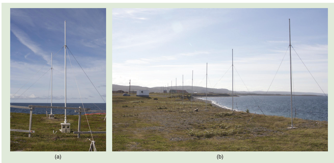
Figure 4: (a) A two-element transmitter array and (b) a 12-element receiver array at Argentia, Newfoundland, and Labrador.
