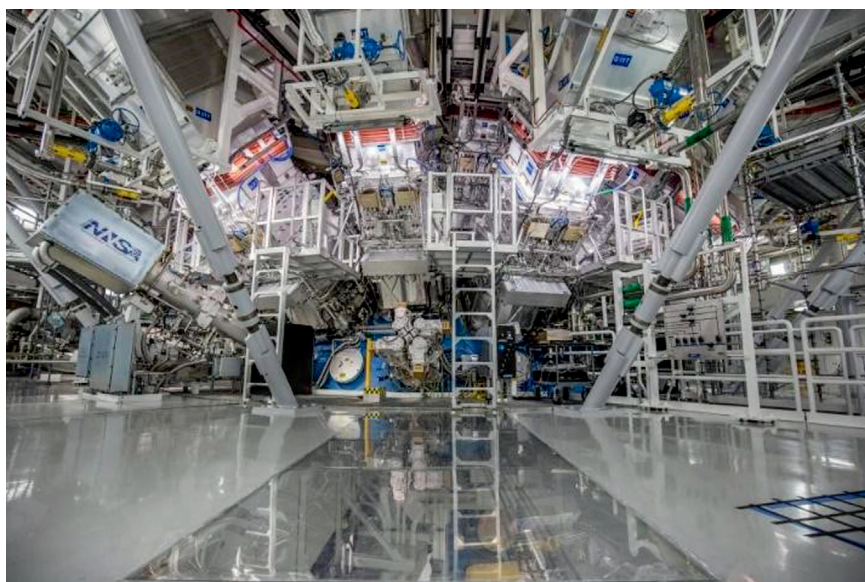
Figure 1: The target chamber of LLNL’s National Ignition Facility, where 192 laser beams delivered more than 2 million joules of ultraviolet energy to a tiny fuel pellet to create fusion ignition. [Source: Reproduced as governed by the permissions of the Creative Commons Copyright License ( www.creativecommons.org/licenses/by-nc-sa/4.0/ ); ( www.llnl.gov/copyright-and-reuse )].
